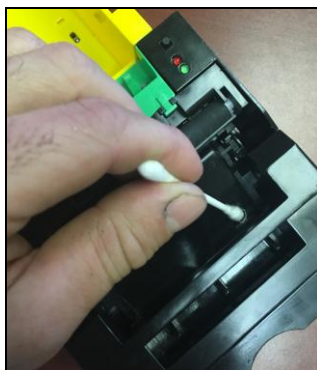
Figure 44: Clean paper guide sensor using a cotton swab
