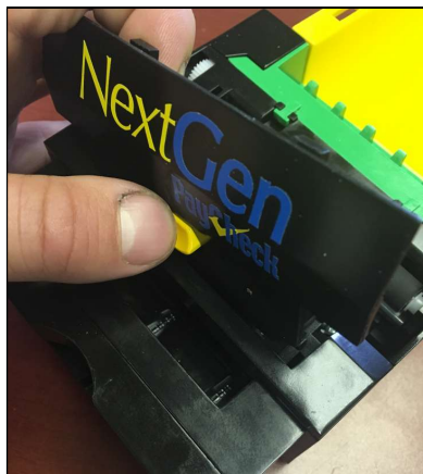
Figure 41: Remove top paper guide
