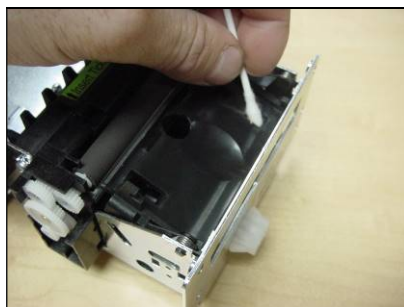
Figure 42: Clean paper guide sensor using cotton swab
