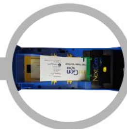
Enclosure opens to the paper path
