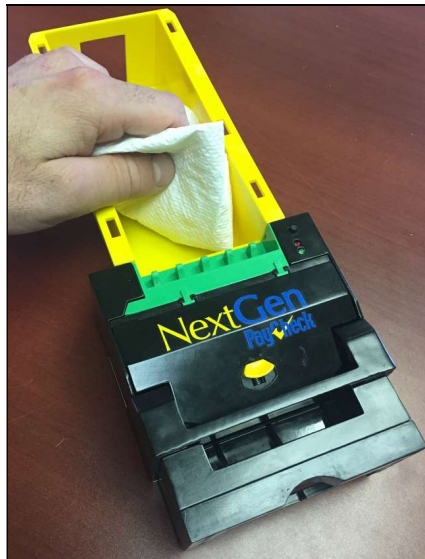
Figure 40: Remove excess dust
