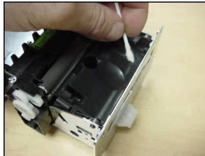
Figure 42: Clean paper guide sensor using cotton swab
