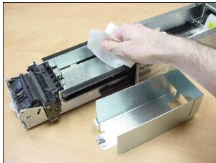
Figure 37: Remove excess dust
