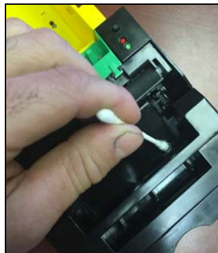
Figure 45: Clean paper guide sensor using a cotton swab
