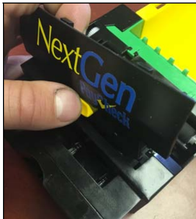
Figure 42: Remove top paper guide
