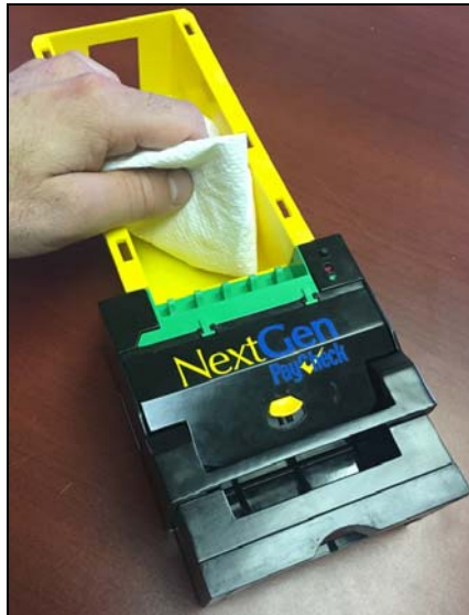
Figure 41: Remove excess dust
