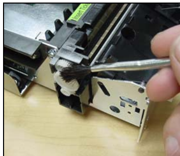
Figure 43: Remove dust from gears using brush
