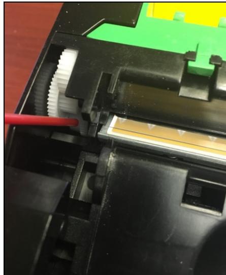
Figure 43: Clear dust off gears using compressed air
