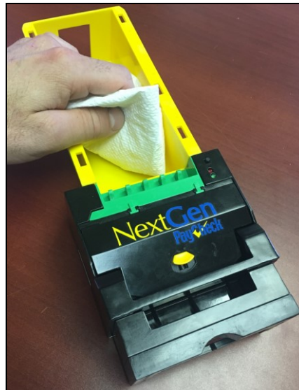
Figure 38: Remove excess dust
