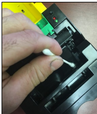
Figure 42: Clean paper guide sensor using a cotton swab
