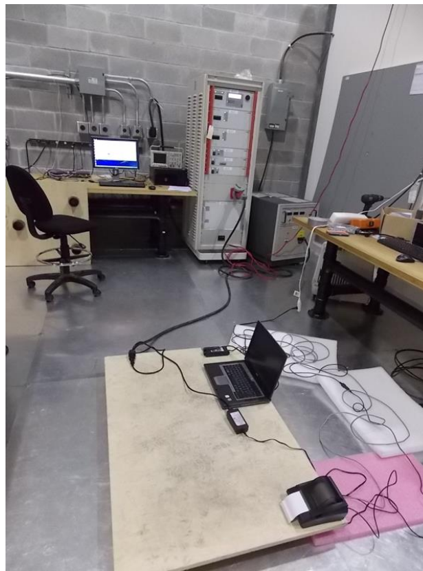
Figure 7.6-1: Voltage dips and voltage interruptions setup photo
