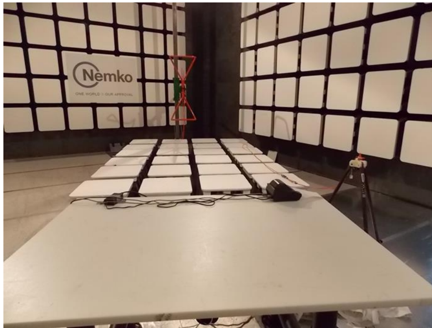
Figure 7.2-1: Continuous RF electromagnetic field disturbances, setup photo (swept test)
