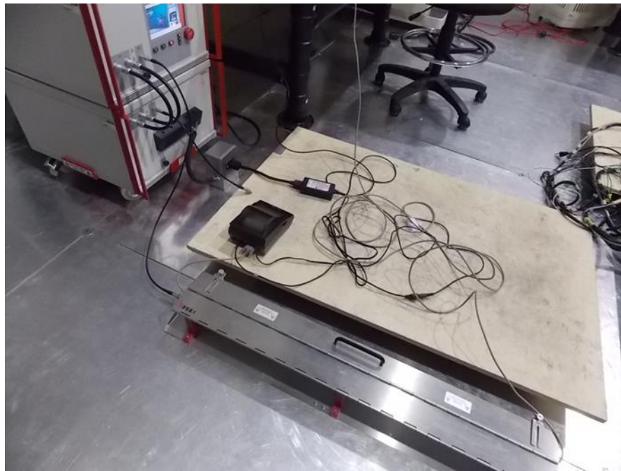
Figure 7.3-1: Electrical fast transients/burst setup photo
