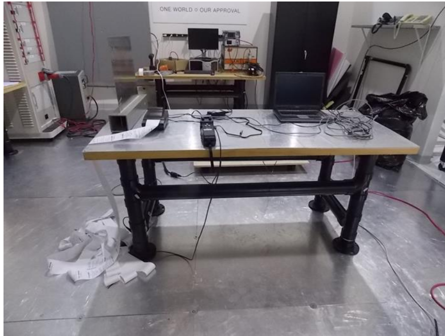
Figure 7.1-1: ESD setup photo
