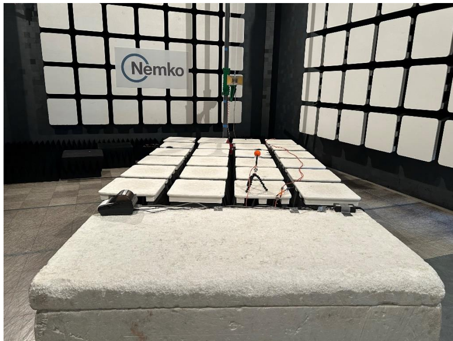
Figure 7.2-4: Continuous RF electromagnetic field disturbances, setup photo (spot test) [2024 assessment]
