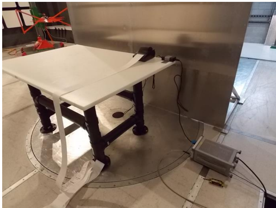
Figure 7.2-6: Conducted emissions – from AC mains power ports setup photo
