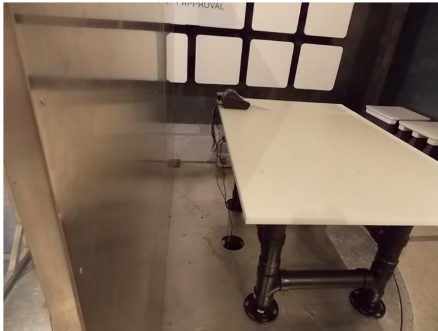
Figure 7.2-5: Conducted emissions – from AC mains power ports setup photo
