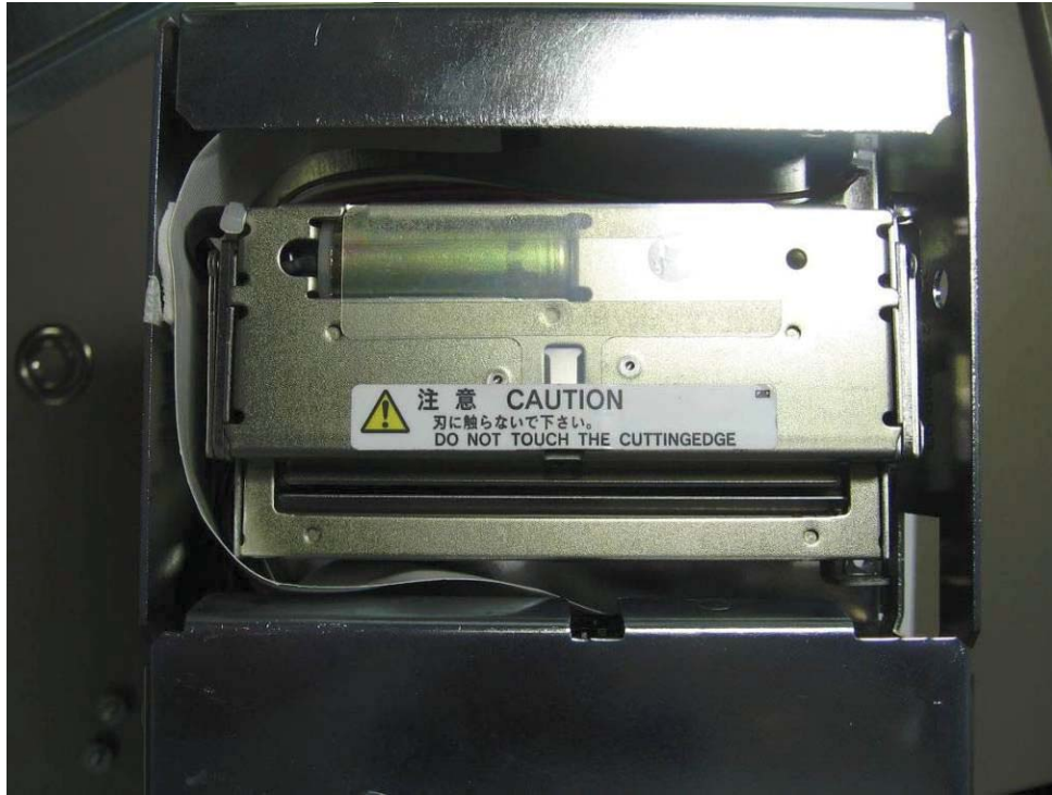
Photo 3 – Motor/Cutter Assembly (For model H/S Kiosk™ “C” and H/S Kiosk™ “V”)
